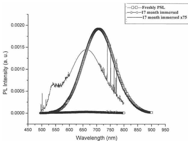
FIGURE 5. PL spectra taken at 10 K for sample S4 at different oxidation degrees. Spectrum 1 for a freshly PSL and spectrum 2 for a sample keep for 17 months in saturated vapor water conditions.
